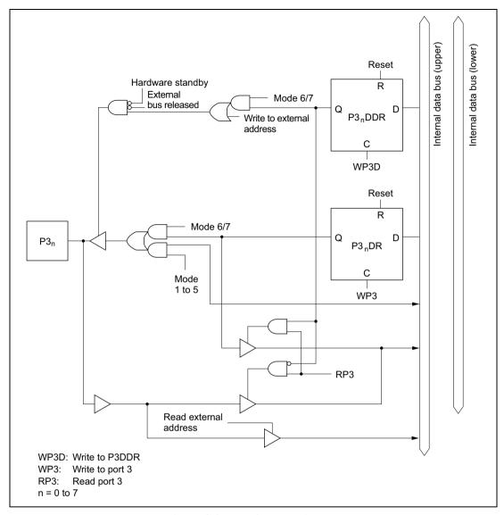
Figure C.3 Port 3 Block Diagram
