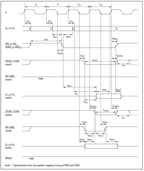
Figure 21.17 DRAM Bus Timing (Read/Write)
