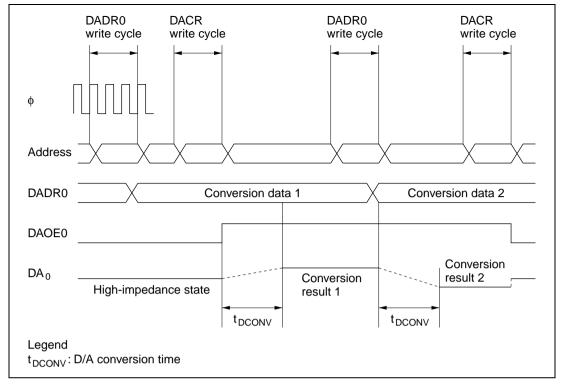
Figure 16.2 Example of D/A Converter Operation
