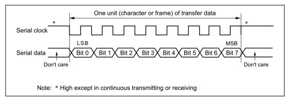
Figure 13.14 Data Format in Synchronous Communication
