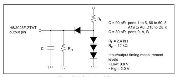
Figure 21.6 Output Load Circuit
