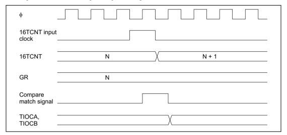
Figure 9.20 Output Compare Output Timing
