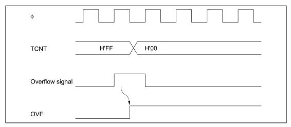
Figure 12.6 Timing of Setting of OVF
