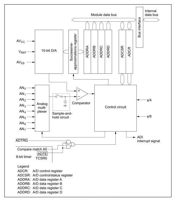
Figure 15.1 A/D Converter Block Diagram
