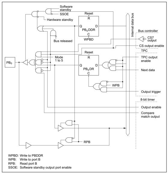
Figure C.11 (a) Port B Block Diagram (Pin PB<sub>0</sub>)
