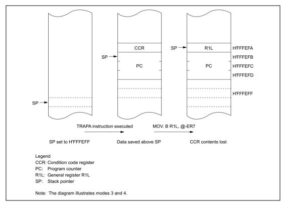
Figure 4.7 Operation when SP Value is Odd
