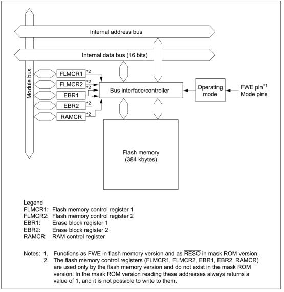
Figure 18.1 Block Diagram of Flash Memory
