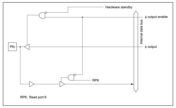
Figure C.6 (g) Port 6 Block Diagram (Pin P67)
