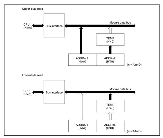
Figure 15.2 A/D Data Register Access Operation (Reading H'AA40)
