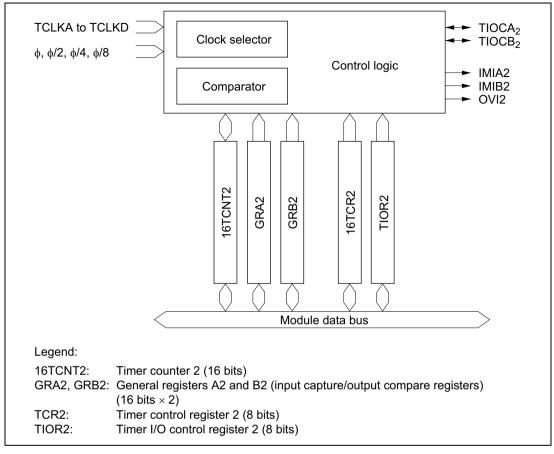
Figure 9.3 Block Diagram of Channel 2
