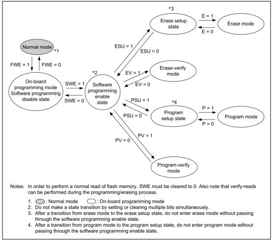
Figure 18.9 FLMCR1 Bit Settings and State Transitions
