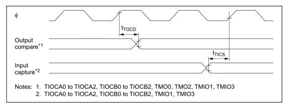
Figure 21.21 Timer Input/Output Timing
