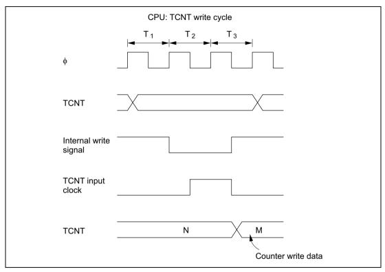
Figure 12.8 Contention between TCNT Write and Count up
