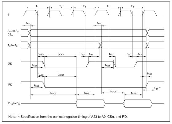
Figure 21.14 Burst ROM Access Timing: Two-State Access
