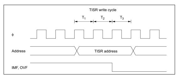
Figure 9.36 Timing of Clearing of Status Flags
