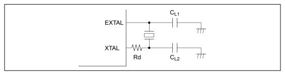
Figure 19.2 Connection of Crystal Resonator (Example)
