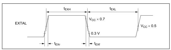
Figure 19.6 External Clock Input Timing
