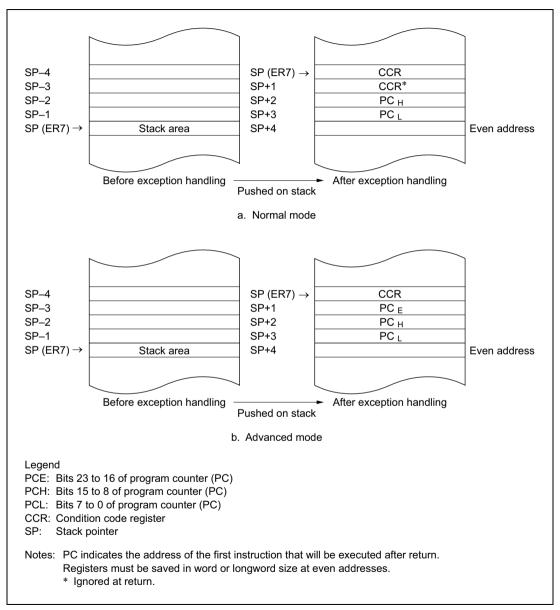
Figure 4.6 Stack after Completion of Exception Handling
