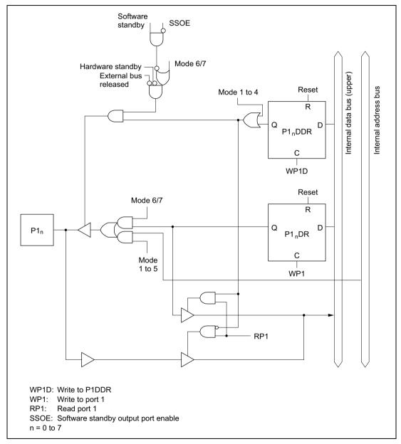
Figure C.1 Port 1 Block Diagram
