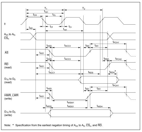
Figure 21.11 Basic Bus Cycle: Two-State Access
