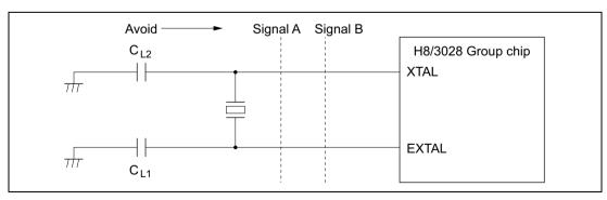
Figure 19.4 Oscillator Circuit Block Board Design Precautions
