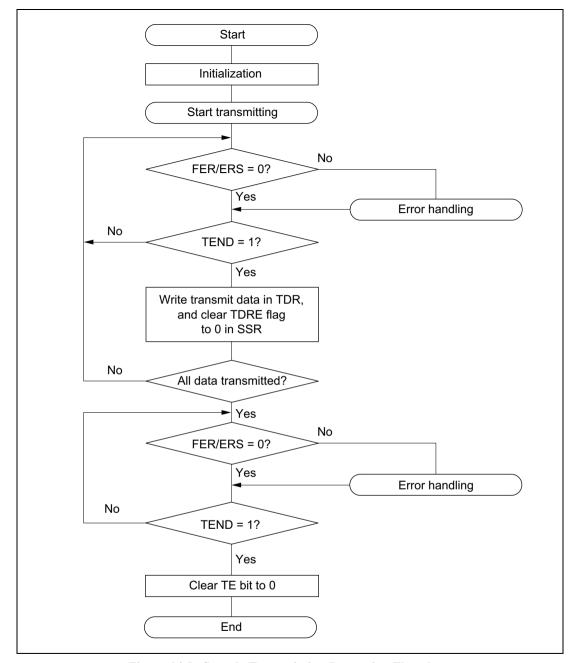
Figure 14.5 Sample Transmission Processing Flowchart
