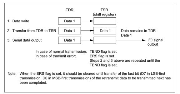
Figure 14.6 Relation Between Transmit Operation and Internal Registers
