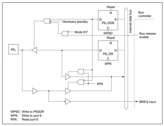
Figure C.6 (b) Port 6 Block Diagram (Pin P6<sub>1</sub>)
