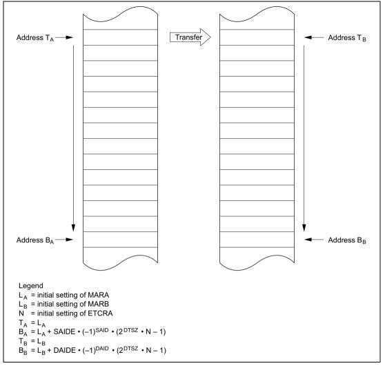
Figure 7.8 Operation in Normal Mode
