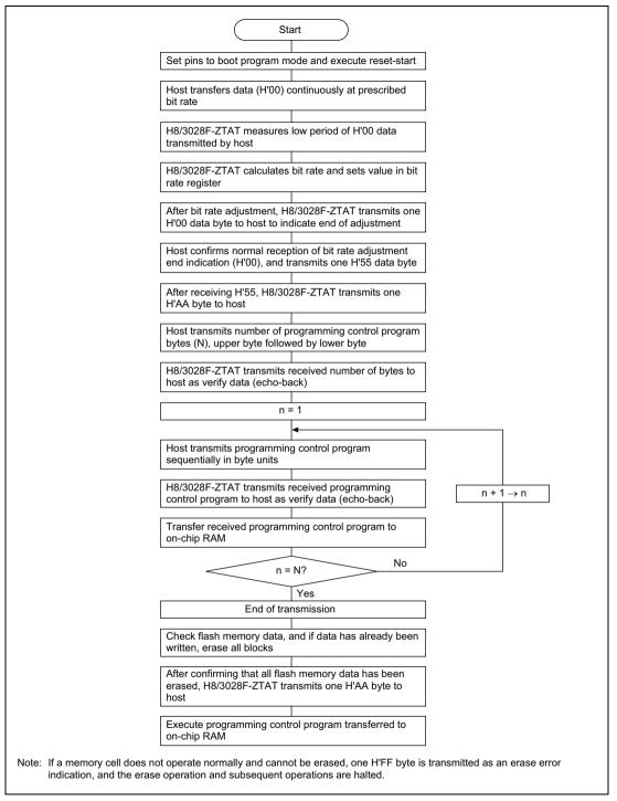
Figure 18.6 Boot Mode Execution Procedure
