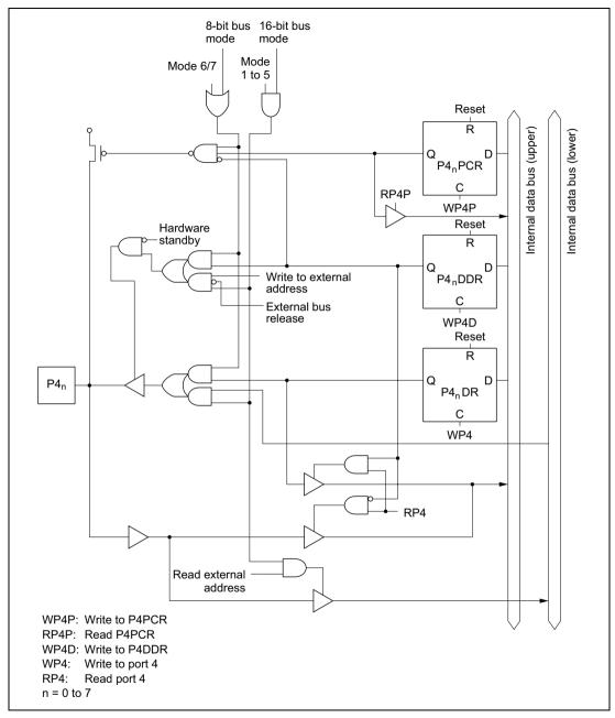
Figure C.4 Port 4 Block Diagram
