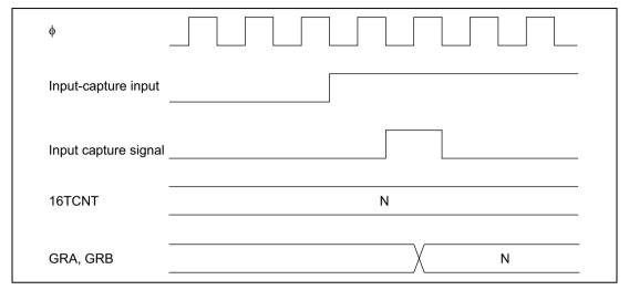
Figure 9.23 Input Capture Signal Timing
