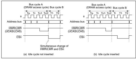
Figure 6.45 Example of Idle Cycle Operation (3) (HWR/LWR Used as UCAS/LCAS)
