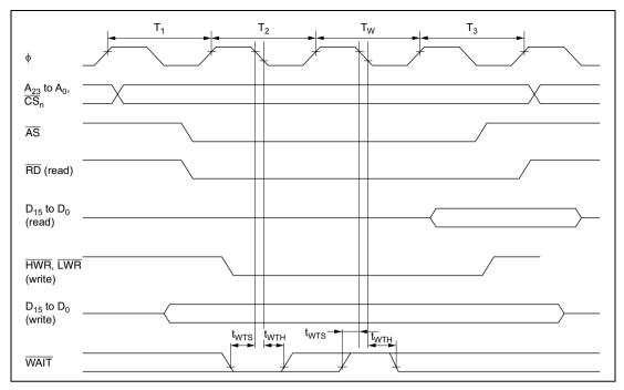
Figure 21.13 Basic Bus Cycle: Three-State Access with One Wait State
