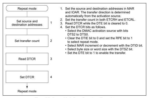
Figure 7.7 Repeat Mode Setup Procedure (Example)
