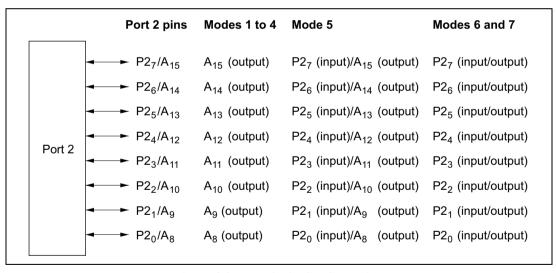
Figure 8.2 Port 2 Pin Configuration
