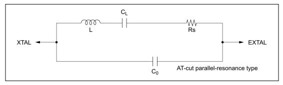
Figure 19.3 Crystal Resonator Equivalent Circuit
