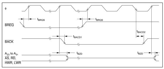
Figure 21.16 Bus-Release Mode Timing
