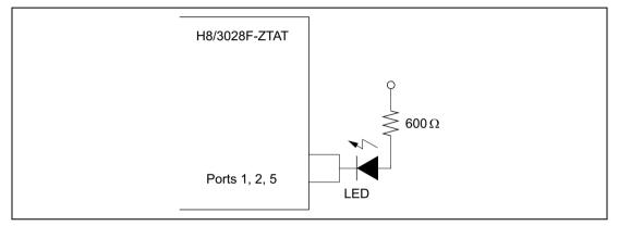
Figure 21.5 Sample LED Circuit
