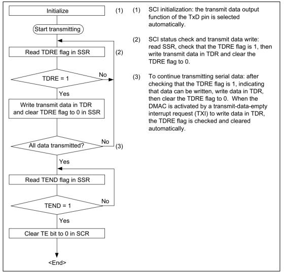
Figure 13.16 Sample Flowchart for Serial Transmitting
