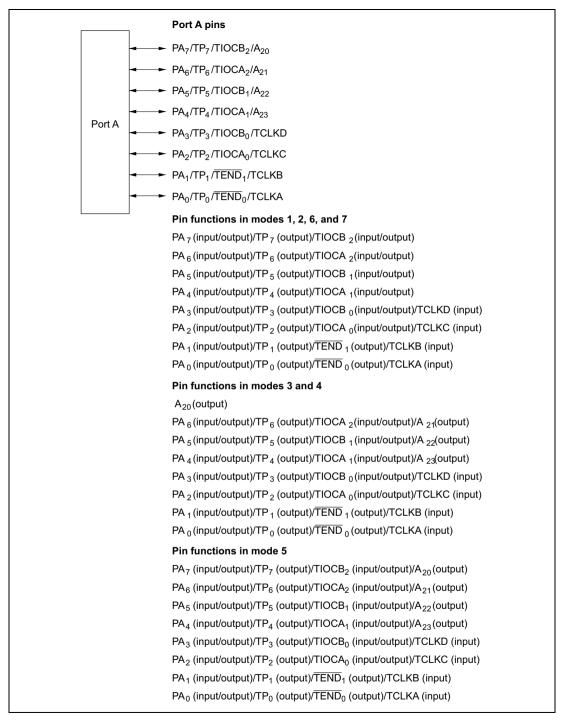
Figure 8.10 Port A Pin Configuration
