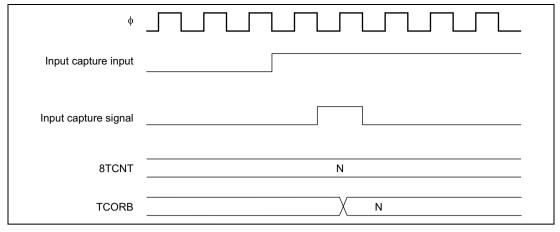
Figure 10.13 Timing of Input Capture Input Signal
