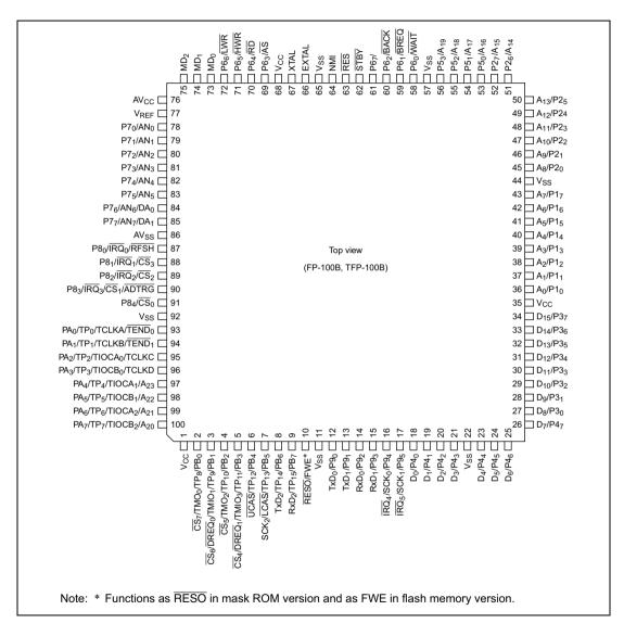
Figure 1.2 Pin Arrangement (FP-100B or TFP-100B, Top View)
