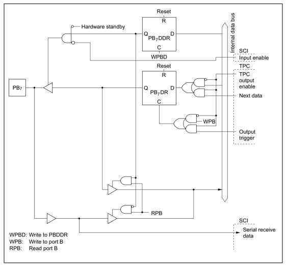
Figure C.11 (h) Port B Block Diagram (Pin PB7)
