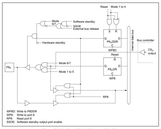
Figure C.8 (e) Port 8 Block Diagram (Pin P84)
