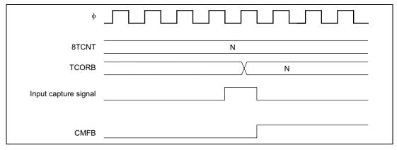
Figure 10.15 CMFB Flag Setting Timing when Input Capture Occurs
