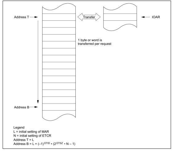
Figure 7.2 Operation in I/O Mode
