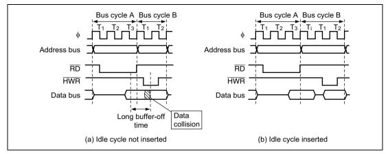
Figure 6.44 Example of Idle Cycle Operation (2) (ICIS0 = 1)
