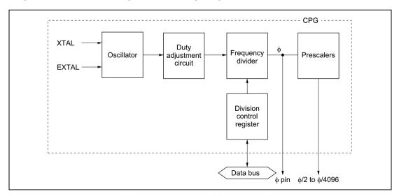
Figure 19.1 Block Diagram of Clock Pulse Generator
