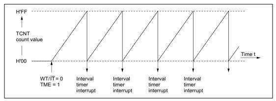
Figure 12.5 Interval Timer Operation
