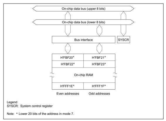
Figure 17.1 RAM Block Diagram
