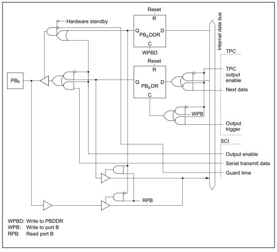
Figure C.11 (g) Port B Block Diagram (Pin PB<sub>6</sub>)
