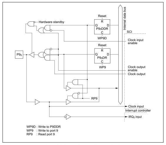
Figure C.9 (f) Port 9 Block Diagram (Pin P95)
