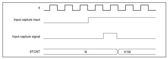
Figure 10.12 Timing of Clear by Input Capture
