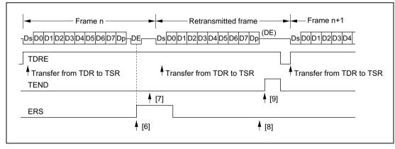
Figure 14.13 Retransmission in SCI Transmit Mode
