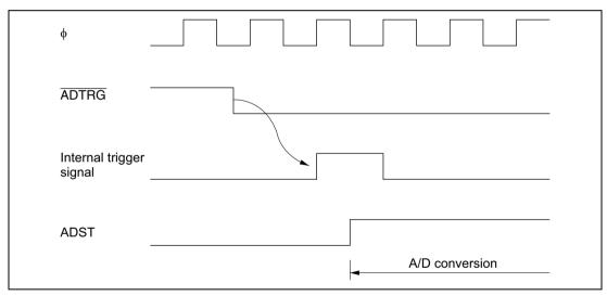
Figure 15.6 External Trigger Input Timing
