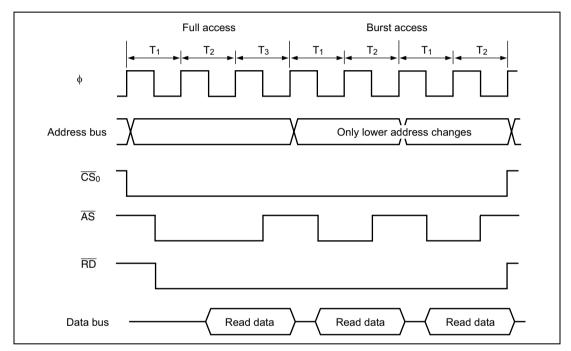
Figure 6.42 Example of Burst ROM Access Timing
