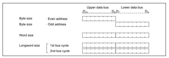
Figure 6.8 Access Sizes and Data Alignment Control (16-Bit Access Area)
