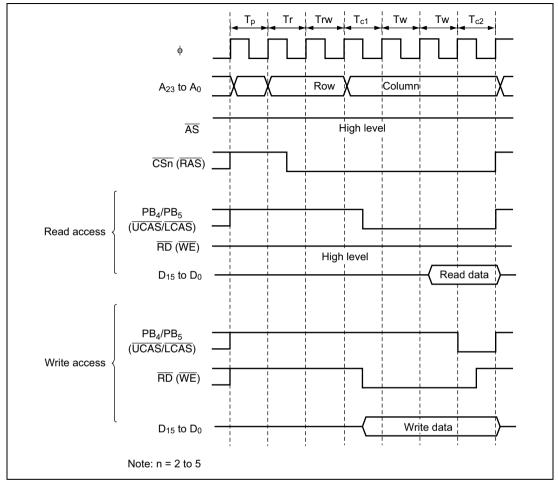
Figure 6.20 Example of Wait State Insertion Timing (CSEL = 0)
