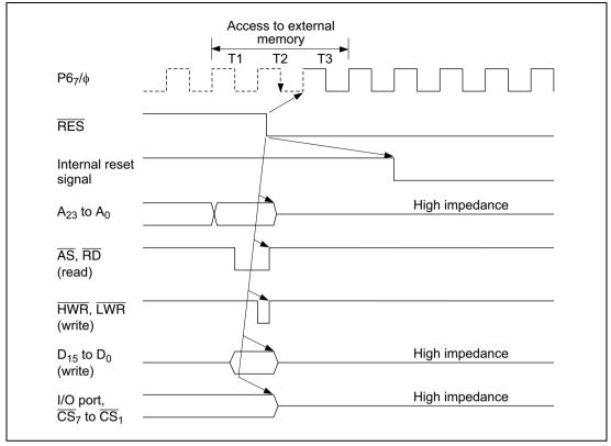
Figure D.3 Reset during Memory Access (Mode 5)
