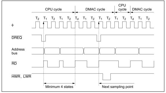
Figure 7.16 Timing of DMAC Activation by Falling Edge of DREQ in Normal Mode
