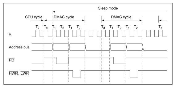
Figure 7.24 Timing of Cycle-Steal Transfer in Sleep Mode
