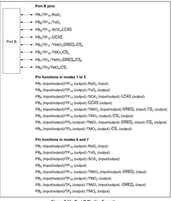
Figure 8.11 Port B Pin Configuration
