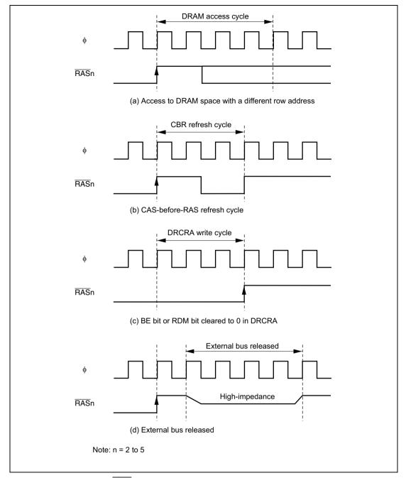
Figure 6.24 RASn Negation Timing when RAS Down Mode is Selected
