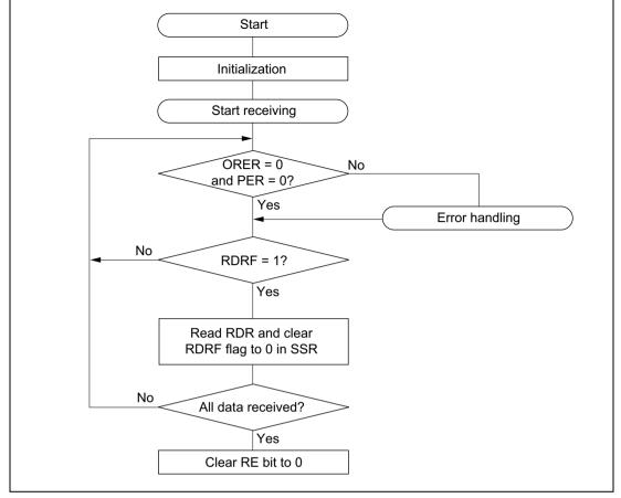
Figure 14.8 Sample Reception Processing Flowchart
