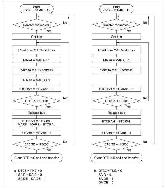
Figure 7.11 Block Transfer Mode Flowcharts (Examples)
