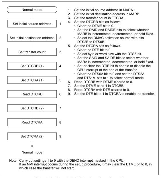
Figure 7.9 Normal Mode Setup Procedure (Example)
