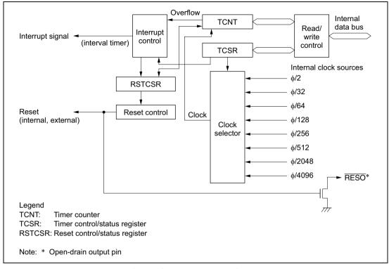
Figure 12.1 WDT Block Diagram
