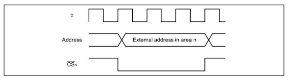
Figure 6.4  $\overline{CS}$ n Signal Output Timing (n = 0 to 7)
