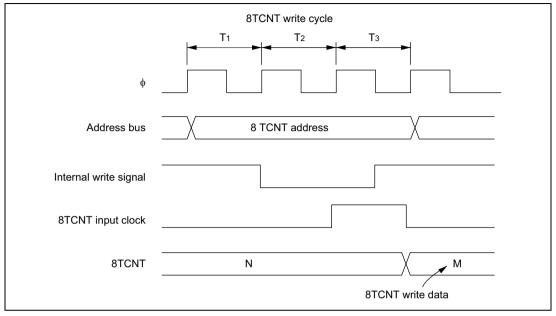
Figure 10.19 Contention between 8TCNT Write and Increment
