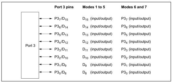
Figure 8.3 Port 3 Pin Configuration
