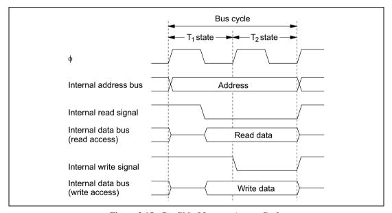
Figure 2.15 On-Chip Memory Access Cycle
