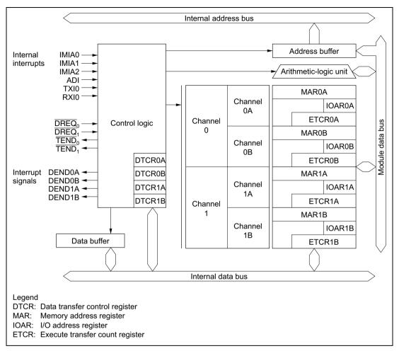
Figure 7.1 Block Diagram of DMAC
