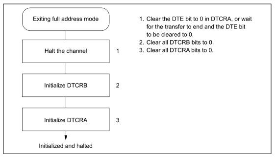
Figure 7.23 Procedure for Exiting Full Address Mode (Example)
