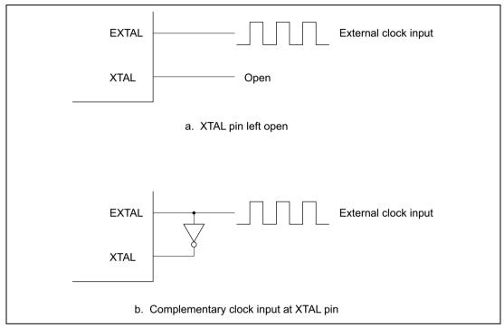
Figure 19.5 External Clock Input (Examples)
