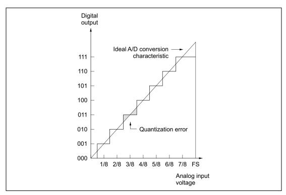
Figure 15.9 A/D Converter Accuracy Definitions (1)
