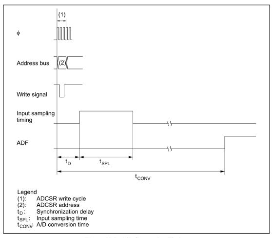
Figure 15.5 A/D Conversion Timing
