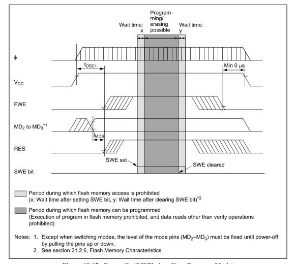
Figure 18.17 Power-On/Off Timing (User Program Mode)
