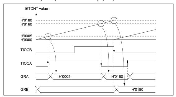
Figure 9.22 Input Capture (Example)
