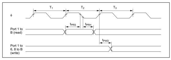
Figure 21.20 TPC and I/O Port Input/Output Timing
