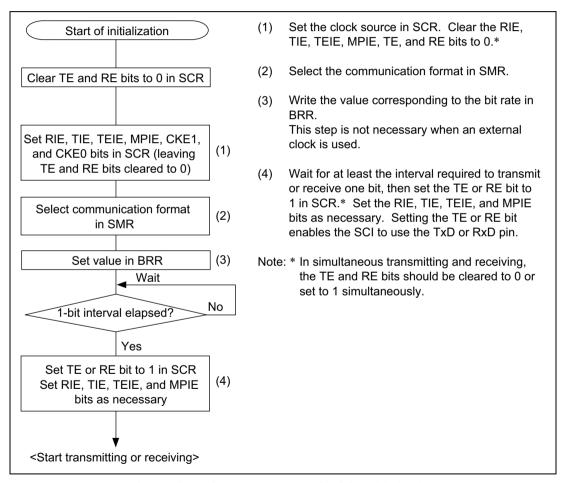
Figure 13.15 Sample Flowchart for SCI Initialization
