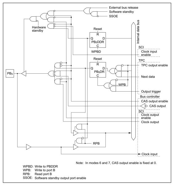
Figure C.11 (f) Port B Block Diagram (Pin PB<sub>5</sub>)
