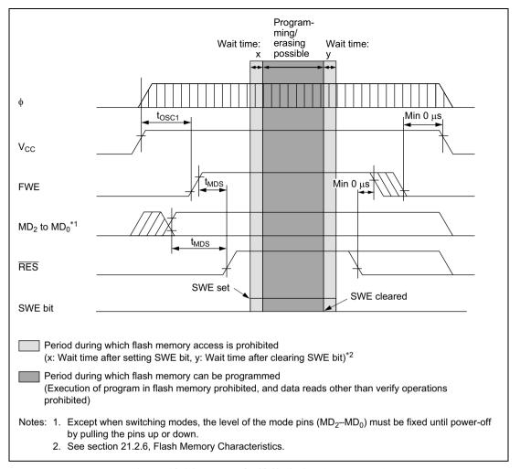
Figure 18.16 Power-On/Off Timing (Boot Mode)
