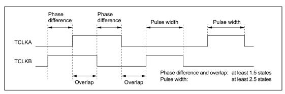
Figure 9.31 Phase Difference, Overlap, and Pulse Width in Phase Counting Mode
