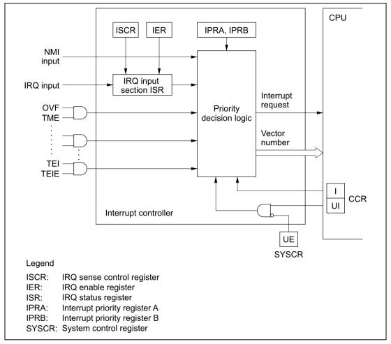
Figure 5.1 Interrupt Controller Block Diagram
