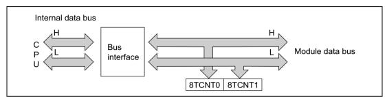
Figure 10.2 8TCNT Access Operation (CPU Writes to 8TCNT, Word)
