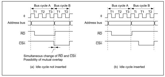
Figure 6.47 Example of Idle Cycle Operation (5)
