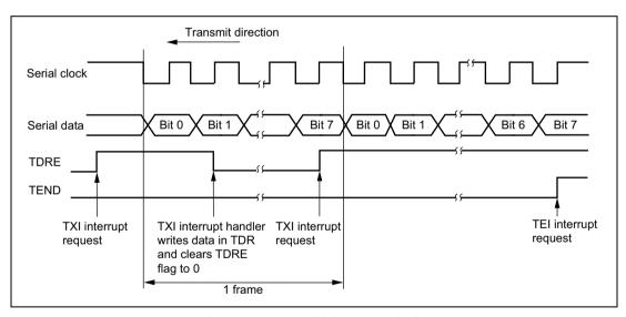
Figure 13.17 Example of SCI Transmit Operation
