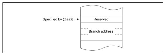
Figure 2.10 Memory-Indirect Branch Address Specification
