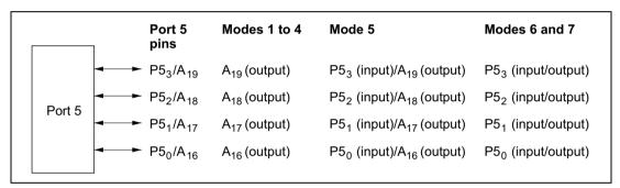
Figure 8.5 Port 5 Pin Configuration
