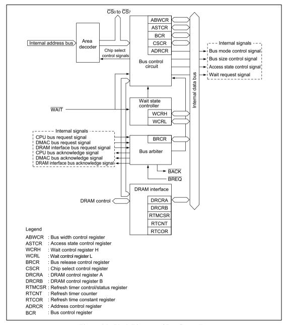
Figure 6.1 Block Diagram of Bus Controller
