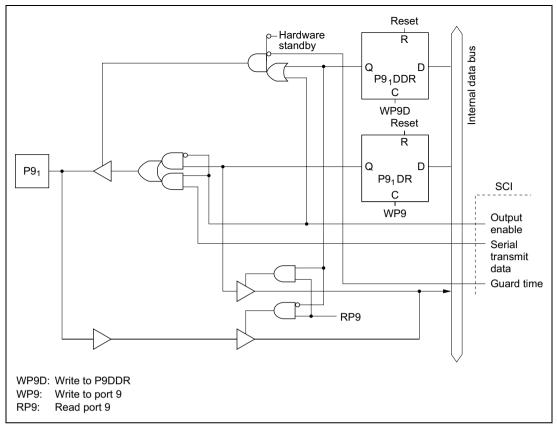
Figure C.9 (b) Port 9 Block Diagram (Pin P9<sub>1</sub>)
