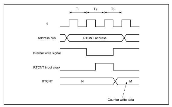
Figure 6.40 Contention between RTCNT Write and Increment
