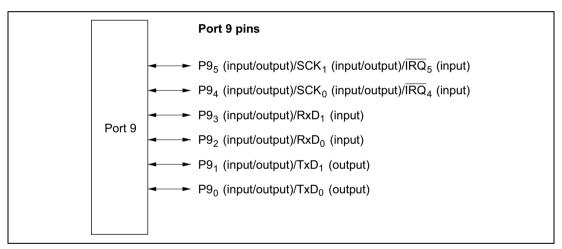
Figure 8.9 Port 9 Pin Configuration
