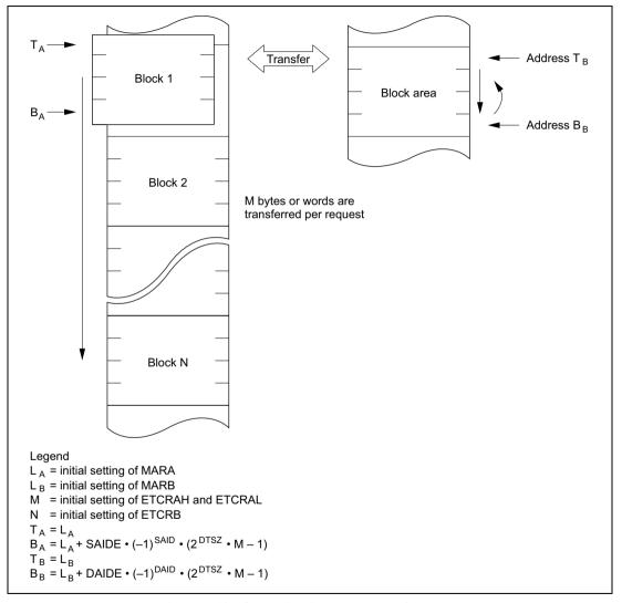
Figure 7.10 Operation in Block Transfer Mode
