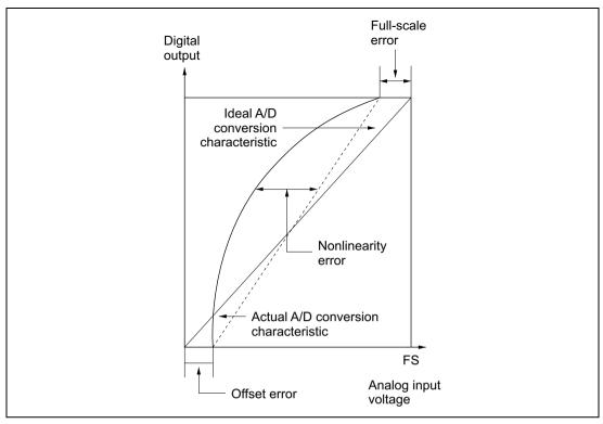
Figure 15.10 A/D Converter Accuracy Definitions (2)
