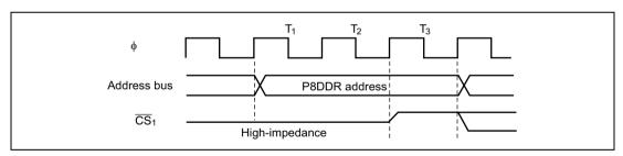
Figure 6.50 DDR Write Timing
