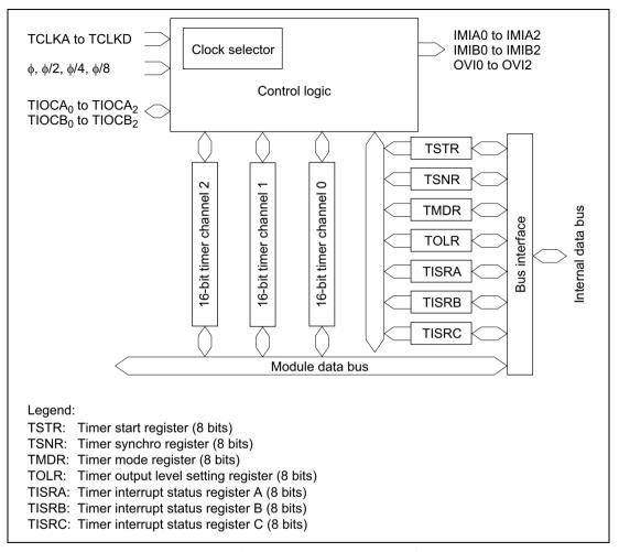
Figure 9.1 16-bit timer Block Diagram (Overall)
