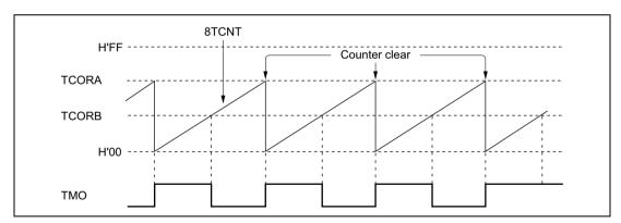
Figure 10.17 Example of Pulse Output
