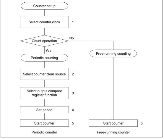
Figure 9.12 Counter Setup Procedure (Example)
