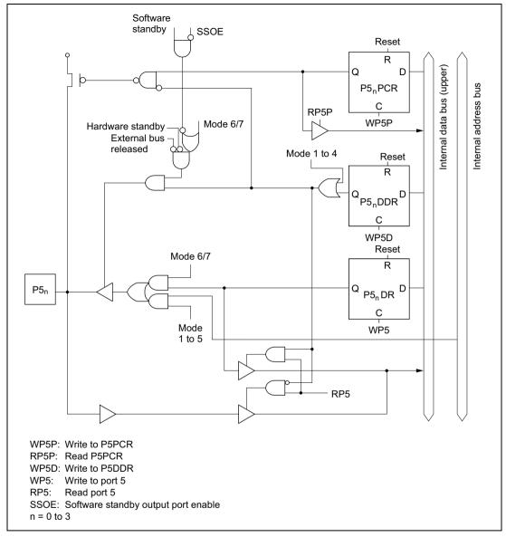
Figure C.5 Port 5 Block Diagram
