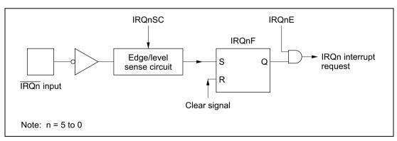
Figure 5.2 Block Diagram of Interrupts IRQ<sub>0</sub> to IRQ<sub>5</sub>
