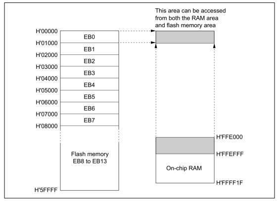
Figure 18.14 Example of RAM Overlap Operation
