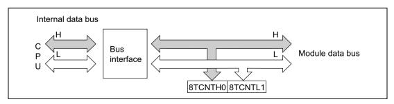
Figure 10.4 8TCNT0 Access Operation (CPU Writes to 8TCNT0, Upper Byte)
