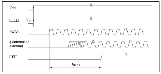
Figure 19.7 External Clock Output Settling Delay Timing
