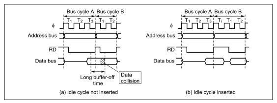
Figure 6.43 Example of Idle Cycle Operation (1) (ICIS1 = 1)
