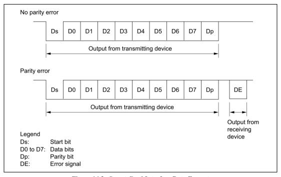
Figure 14.3 Smart Card Interface Data Format
