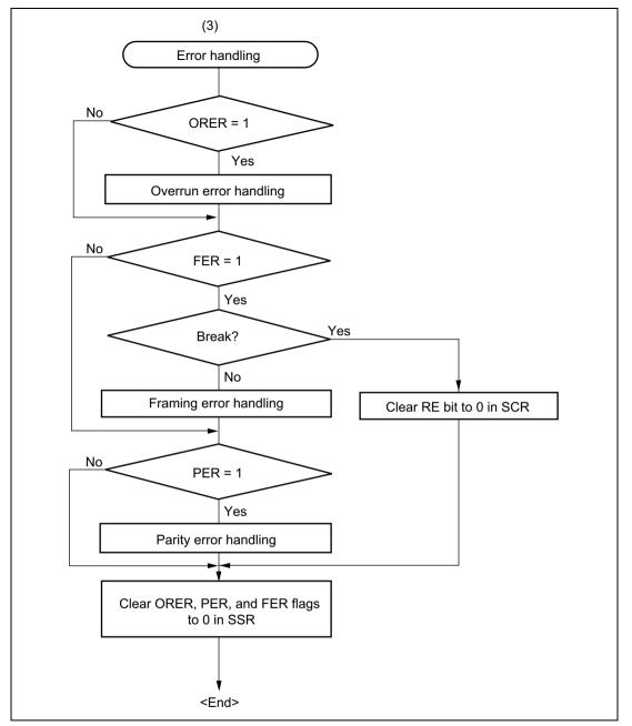
Figure 13.7 Sample Flowchart for Receiving Serial Data (2)
