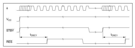
Figure 21.7 Oscillator Settling Timing
