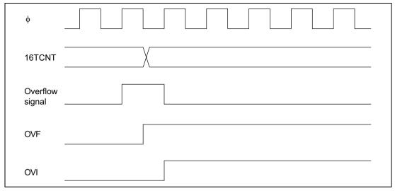
Figure 9.35 Timing of Setting of OVF
