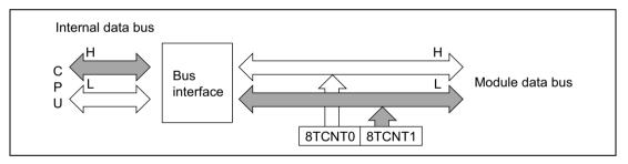
Figure 10.7 8TCNT1 Access Operation (CPU Reads 8TCNT1, Lower Byte)
