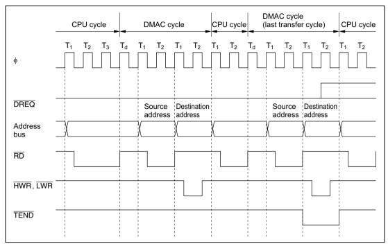
Figure 7.14 Bus Timing of DMA Transfer Requested by Low DREQ Input
