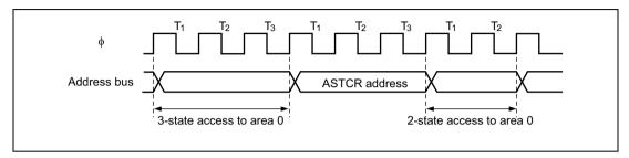
Figure 6.49 ASTCR Write Timing
