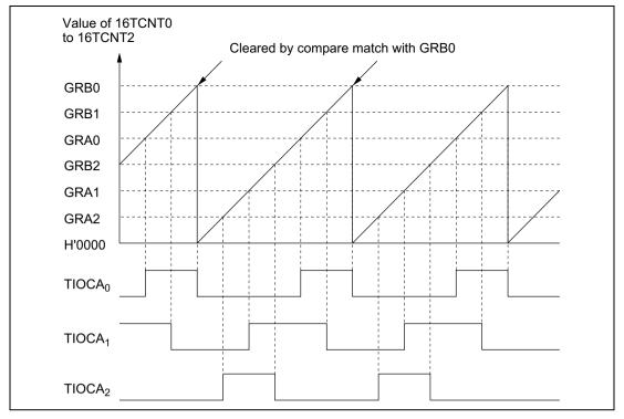
Figure 9.25 Synchronization (Example)
