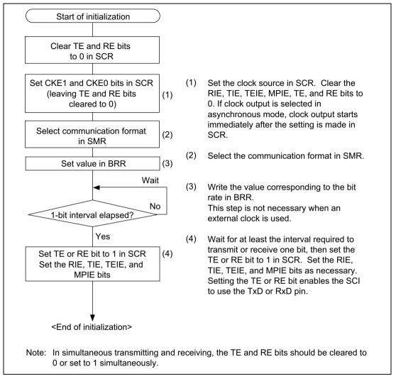
Figure 13.4 Sample Flowchart for SCI Initialization
