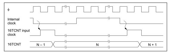
Figure 9.15 Count Timing for Internal Clock Sources
