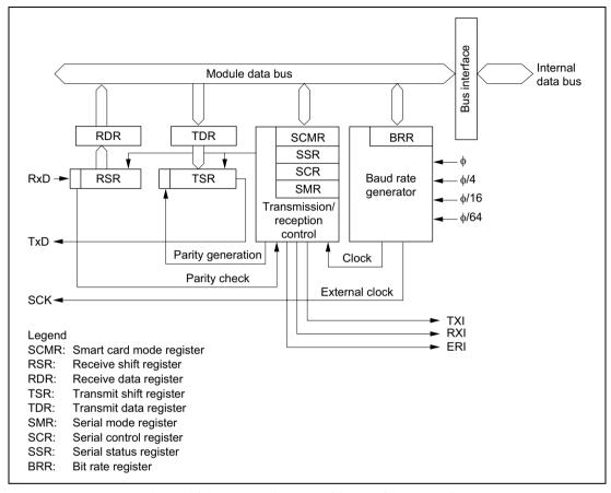
Figure 14.1 Block Diagram of Smart Card Interface
