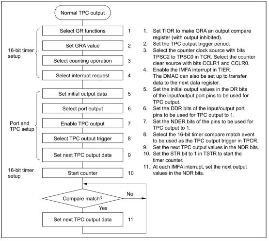
Figure 11.4 Setup Procedure for Normal TPC Output (Example)
